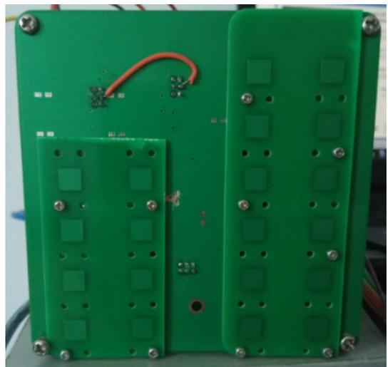
Fig.4 Monopulse motion sensor prototype assembled
