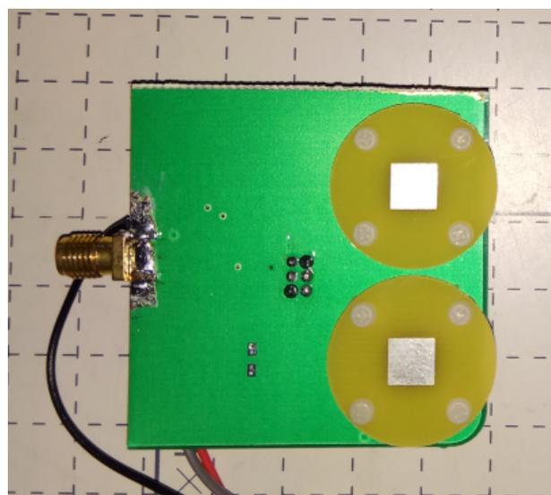
Fig.1 Aperture coupled patch antenna.
