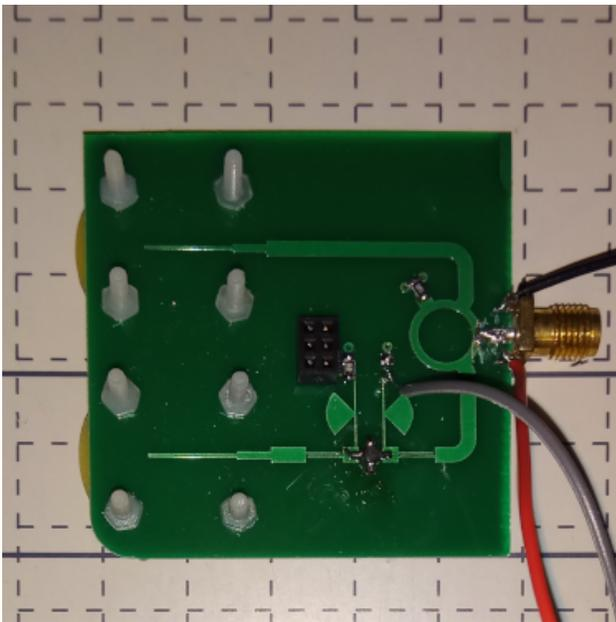
Fig.2 Aperture coupled patch antenna feeding
