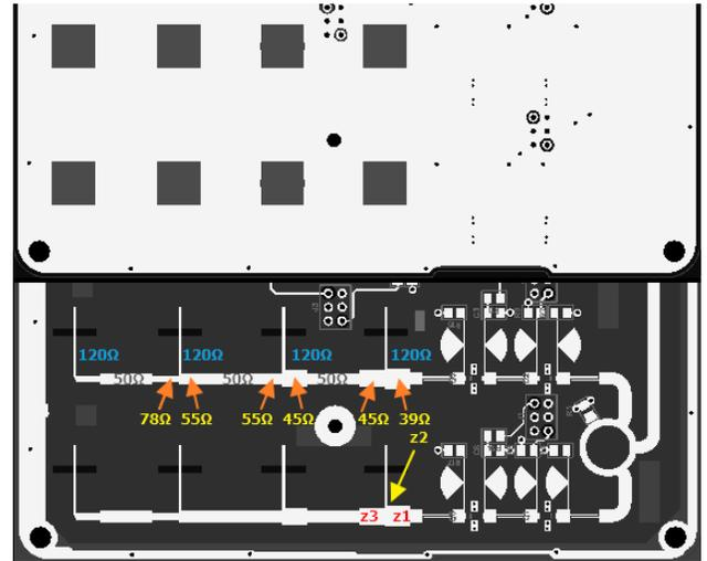
Fig.3 Monopulse motion sensor prototype receiver
